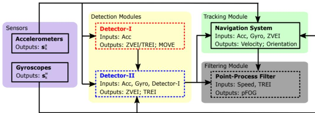
Figure 3: A block diagram of the system used to calculate the pFOG.
