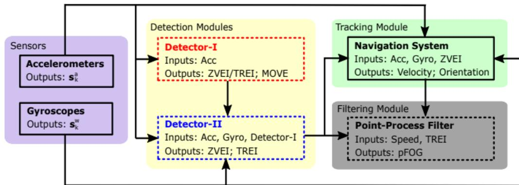
Figure 3: A block diagram of the system used to calculate the pFOG.
