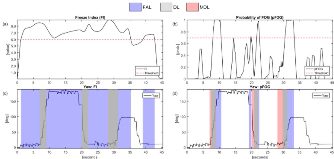
**Figure 5:** (a) Freeze-Index plot with FI-threshold set to 6.0. (b) pFOG plot with  $\sigma_s = 0.29$ . (c) and (d) Yaw angle plot with an overlay of DL, MDL, and FAL. FOG region marked using video data<sup>10</sup>.
